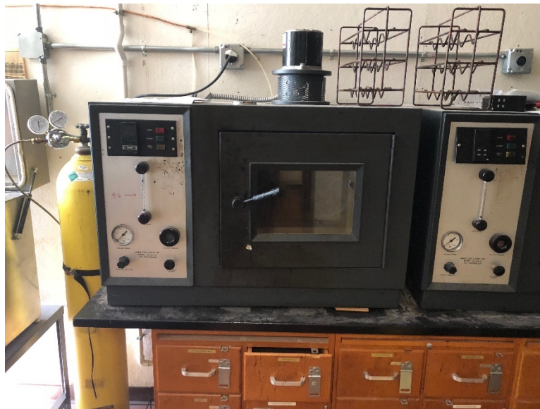
Figure 5-3. The rolling thin-film oven test apparatus
