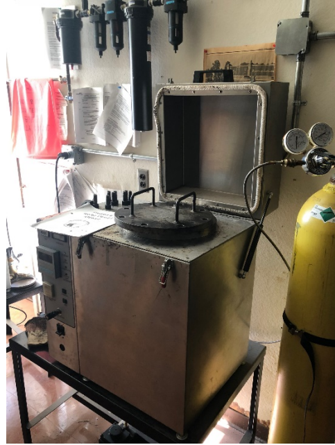
Figure 5-4. The pressure aging vessel (PAV) test apparatus
