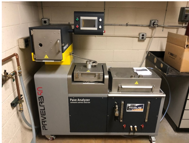
Figure 5-1. The automatic asphalt analyzer used to separate asphalt from the asphalt mixture
