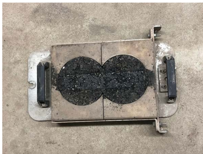
Figure 3-1. The specimen and the cylindrical specimen mounting system
