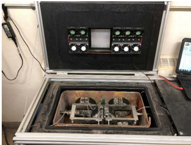
Figure 4-3. DCT test equipment produced by the TestQuip LLC
