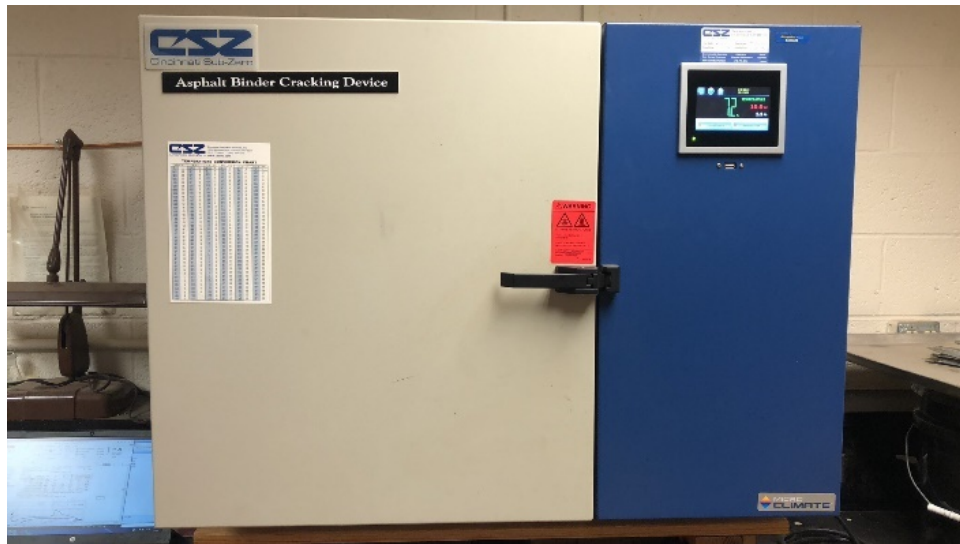
Figure 5-8. The Asphalt Binder Cracking Device (ABCD) test apparatus
