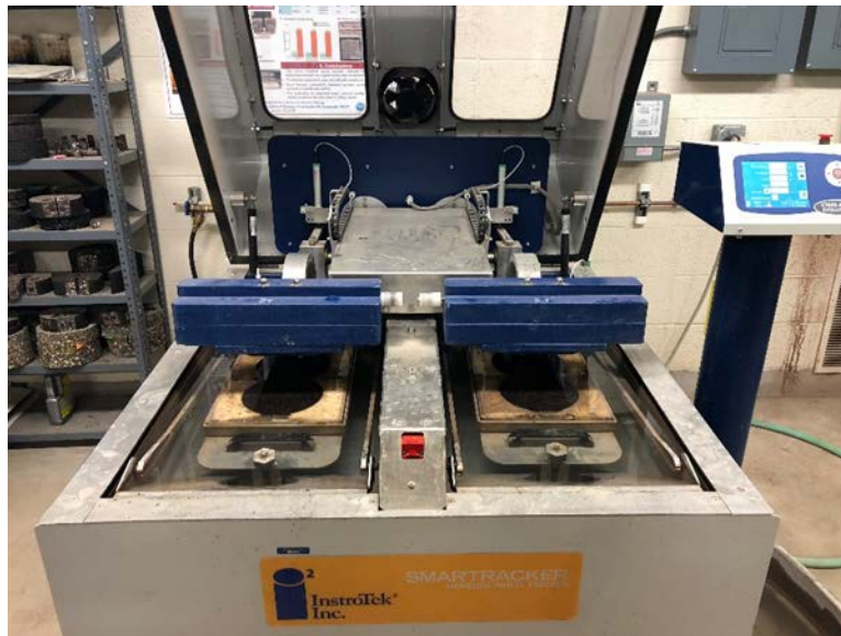
Figure 3-2. The Hamburg Wheel Tracking Device
